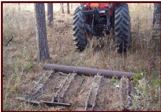
A simple drag designed to disturb the top layer of the soil without breaking the soil.
